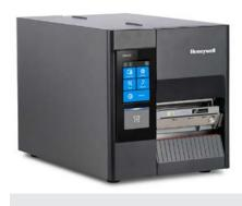
Thanks to a very ergonomic design, the print head can be easily switched out and replaced. The front sensor that ensures accurate printing can also be easily removed to facilitate cleaning and replacement of the rubber roller. The PD45S supports multiple printer command languages such as FP/DP/IPL/ZPL/DPL, one-key installation of printer driver and easy windows configuration.
